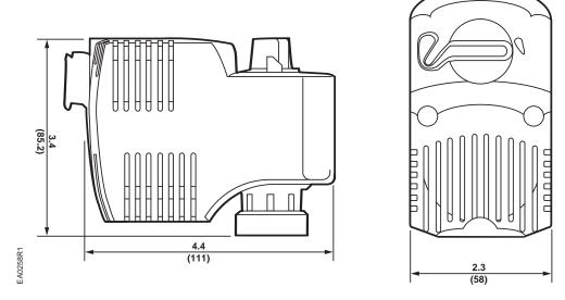
Figure 7. Dimensions of the SFx Series Actuator.
